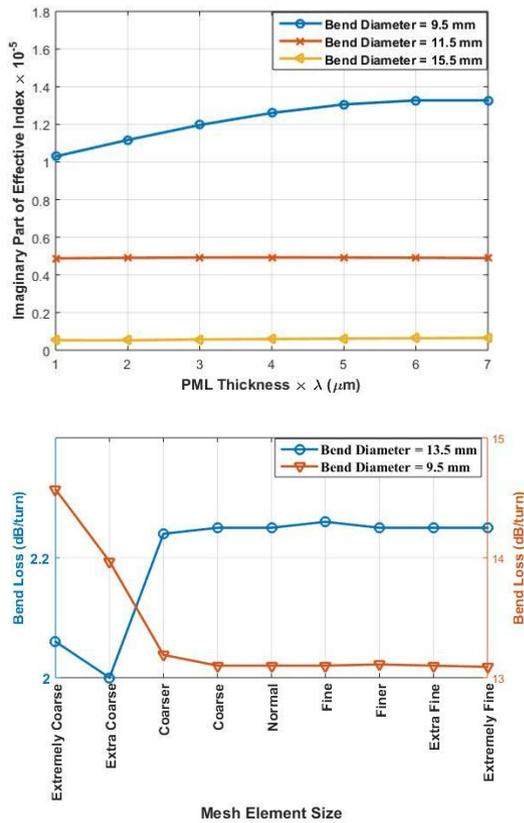
**Fig. 5:** Sensitivity of simulation results with (a) PML thickness and (b) Mesh element size
