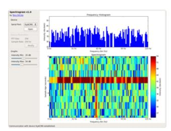
Finally, try changing the sample rate by clicking the Modify button in the Device Parameters group on the left. You can use values from ~150hz to ~9000hz. Notice as the sample rate decreases, both the range of frequencies decreases (at a rate of half the sample rate) and the amount of time to get a new sample increases (because it takes longer to fill the 256 samples for running the FFT).
