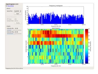
Unfortunately in practice I found trying to detect purrs reliably is quite difficult. The spectrogram to the left shows more typical data, where the movement of the cat against the microphone (or even biting the microphone!) generates a lot of noise which obscures the purr. The noise unfortunately leads to false positives which make the purr detection unreliable.
