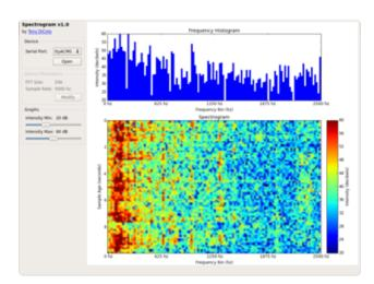
The spectrogram is a powerful tool we'll use in this guide to analyze audio. For now try playing some audio or making noise to see how it's represented on the graphs. For example the picture on the left is showing the spectrogram of audio from the opening of this orchestral piece ().
