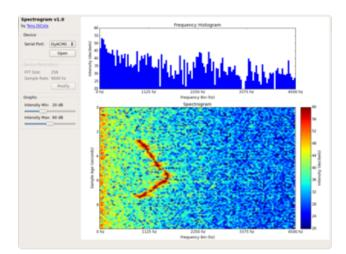
First we need to understand what frequencies make up the sequence of tones to detect. The spectrogram tool from the previous page is the perfect tool for this analysis.
