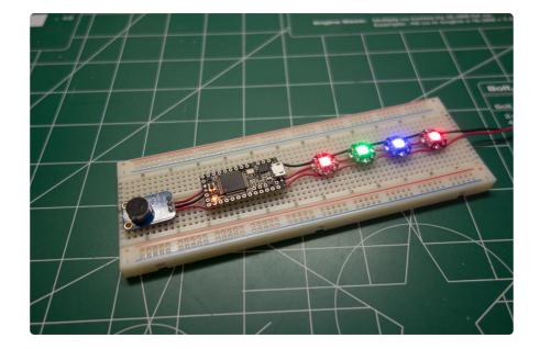
Have you ever wanted to build devices that react to audio, but have been unsure about or even intimidated by analyzing signals? Don't worry! This guide is an overview of applying the Fourier transform, a fundamental tool for signal processing, to analyze signals like audio. I'll show you how I built an audio spectrum analyzer, detected a sequence of tones, and even attempted to detect a cat purr--all with a simple microcontroller, microphone, and some knowledge of the Fourier transform.
